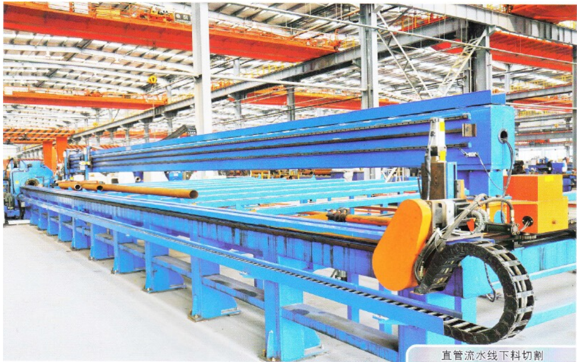
Assembly line of cutting large diameter pipe
