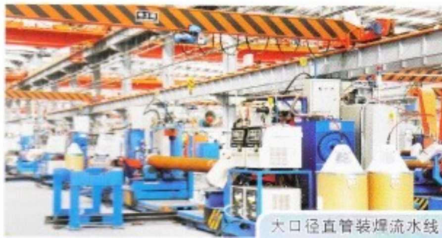
Assembly line of welding large diameter pipe
