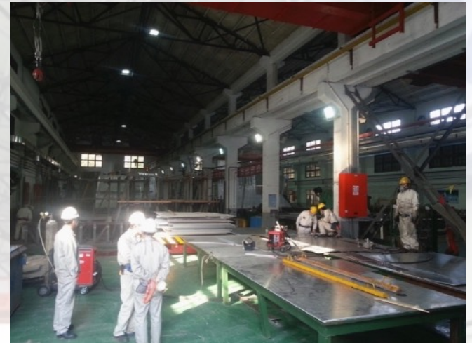
Welding table for bigger plates
