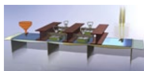
Temporary restraint beams positioned and cavities filled
