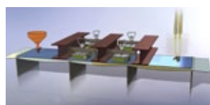
Temporary restraint beams positioned and cavities filled
